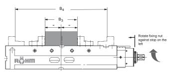
Remove central jaw Fixing nut - stop on the <u>left</u> (spindle rigid) Stroke per jaw: "Z" 53 mm
