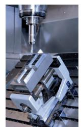
Without additional foundations or special jaws, the RZM centric vice holds the workpiece securely – and does this with a minimal interference contour. The clamping spindle is located very close to the workpiece, creating an effective force flow and providing an extremely rigid clamping. The patented guide system of the jaws makes a very large clamping range possible.
