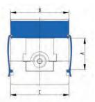
A37 V-jaw SPR, with vertically and horizontally ground-in prisms, hardened, for combination with SGN
