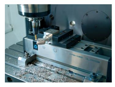
The NC-compact vices from RÖHM are excellently suited for use in single or series production. Different types and constructional lengths enable the optimal adaptation to the work area, workpiece and machining task.
