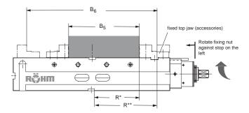
Remove central jaw and movable mounting jaw I. Install fixed mounting jaw (accessory - not in scope of delivery). Fixing nut - stop on the <u>left</u> (spindle rigid) Stroke of moving jaw: "Z" 53 mm
