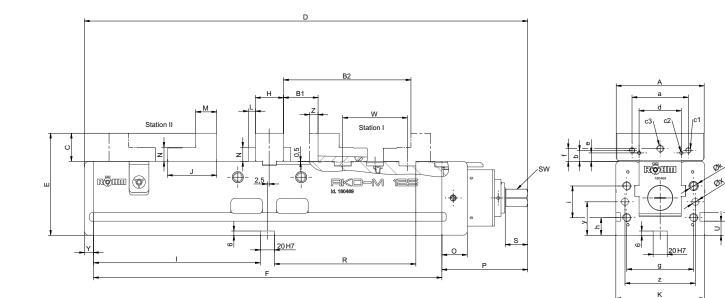
A37 Stepped jaws SB, reversible, with fixing screws
